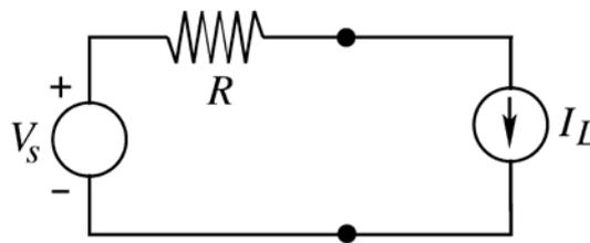
The value of  $I_L$  that maximizes the power absorbed by the constant current load is
