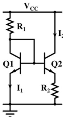
The value of  $R_2$  (in  $\Omega$ ) for which  $I_2=100\text{ }\mu\text{A}$  is \_\_\_\_\_
