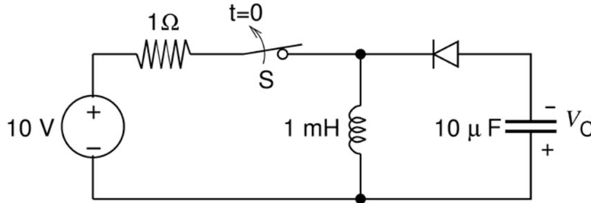
The steady state magnitude of the capacitor voltage  $V_C$  (in volts) is \_\_\_\_\_
