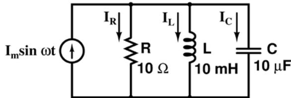
At resonance, the ratio  $|I_L|/|I_R|$ , i.e., the ratio of the magnitudes of the inductor current phasor and the resistor current phasor, is \_\_\_\_\_
